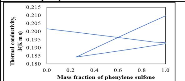
Figure 11. Change in thermal conductivity fluctuate with mass fraction of phenylene sulfone.
