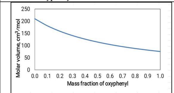
Figure 13. Change in molar volume with mass fraction of oxyphenyl
