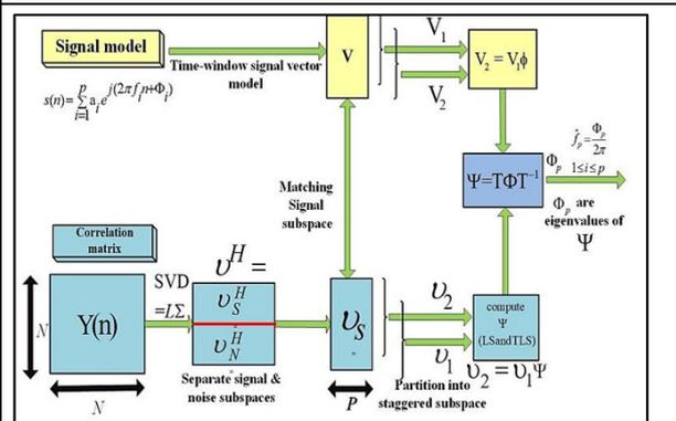
Fig. 4: Steps for application of Adaptive based-TLS-ESPRIT Algorithm for frequency estimation
