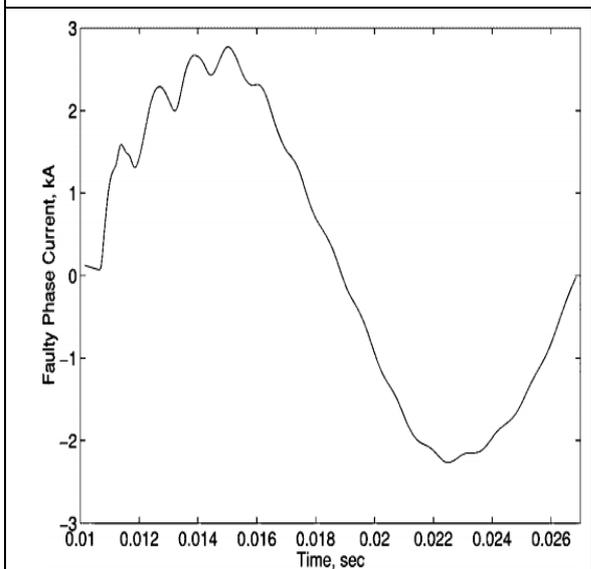
**Figure 4. Current Waveform of the Faulty Phase [17].**
