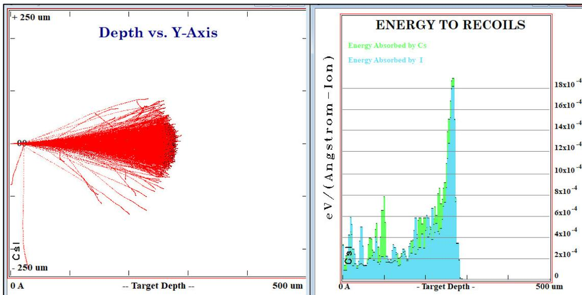
Fig.2.(Left) The range and the tracks of the Proton ion having 6 MeV incident energy inside CsI detector. (Right) same incident ion but the recoil distribution (here one can see both Cs and I atom independently)
