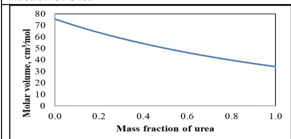
Figure 14. Change in molar volume with mass fraction of Urea
