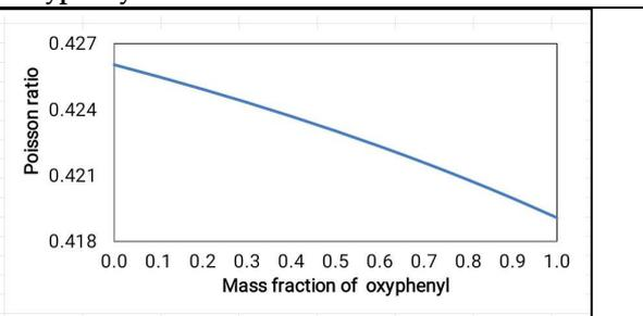
Figure 8. Change in Poisson modulus with mass fraction of oxyphenyl
