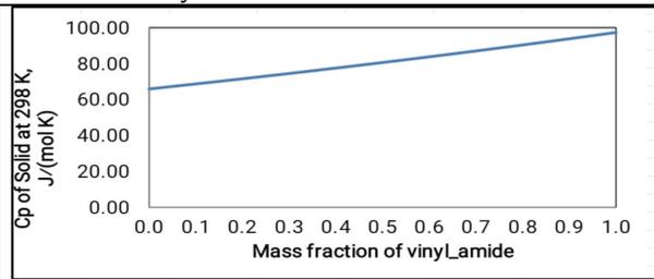
Figure 10. Change in heat capacity with the mass fraction of vinyl amide
