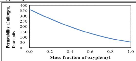
Figure 16. Change in permeability of nitrogen with mass fraction of oxyphenyl
