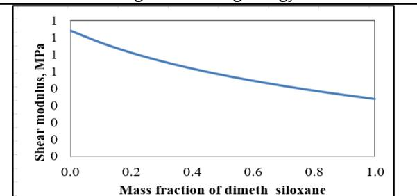
**Figure 6. Change in shear modulus with mass fraction of dimethyl siloxane**
