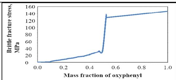
Figure 9. Change in brittle fracture stress with mass fraction oxyphenyl
