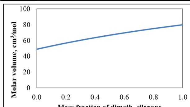
Figure 12. Change in molar volume with mass fraction of dimethyl siloxane
