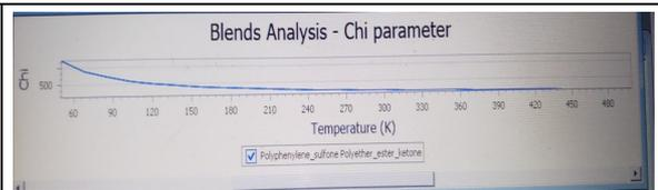
Figure 2. Change in  $\chi$  (chi) value with temperature
