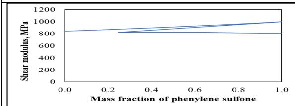
Figure 6. Change in shear modulus with mass fraction of phenylene sulfone.
