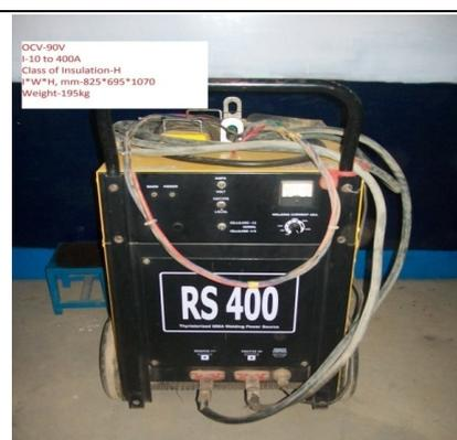
Fig. 7. Welding machine used
