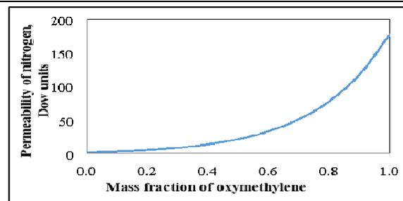
Figure 16. Change in permeability of nitrogen with mass fraction of polyoxymethylene
