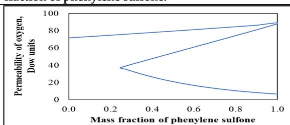
Figure 15. Change in permeability of oxygen with mass fraction of phenylene sulfone
