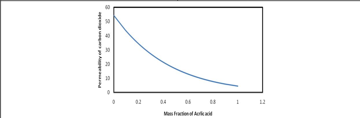
**Figure 5. Change in permeability of carbon dioxide with mass fraction of acrylic acid**
