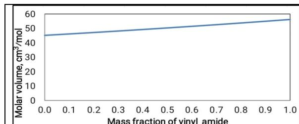
Figure 13. Change in molar volume with the mass fraction of vinyl amide
