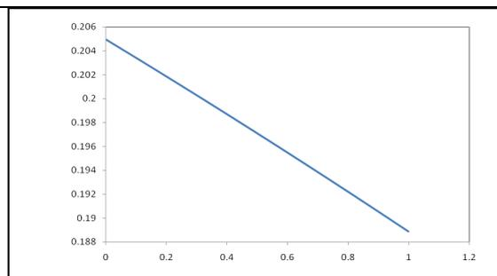
Figure 2. Change in thermal conductivity with mass fraction of acrylic acid
