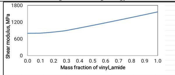
Figure 6. Change in shear modulus with a mass fraction of vinyl amide
