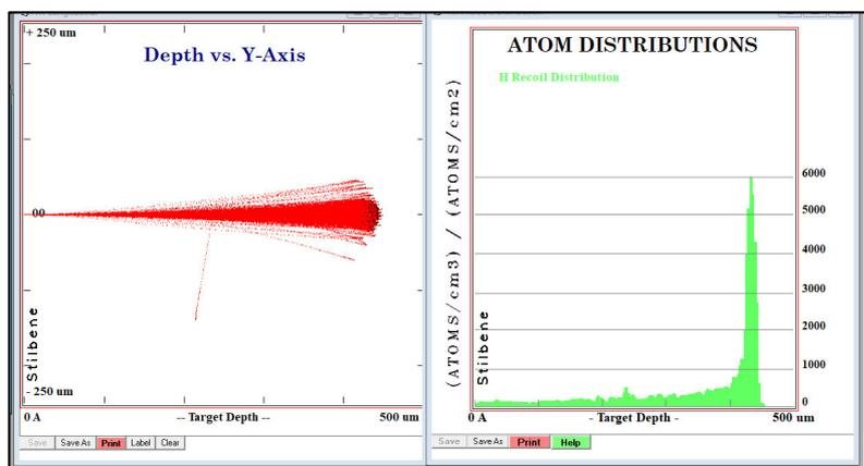
Figure 2: The passage of radiation (proton) inside the scintillator the stilbene. One can see that they will stop in 500um. (right) the recoil distribution inside the stilbene and it is a perfectly sharp distribution towards the end indicates the full energy loss.
