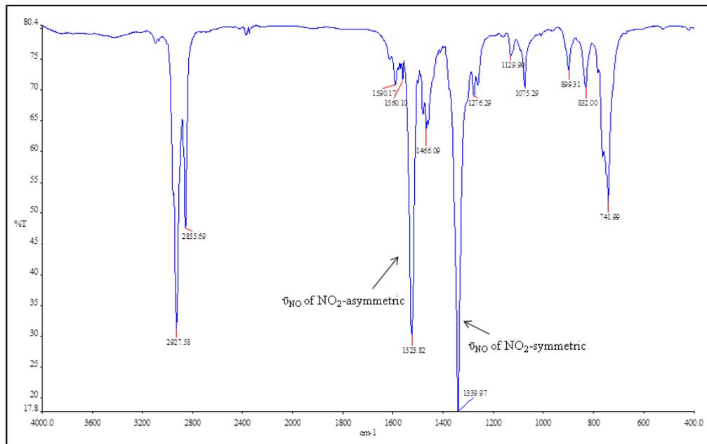
Figure 3. FTIR spectrum of 2,7-dinitro-9,9-dioctylfluorene
