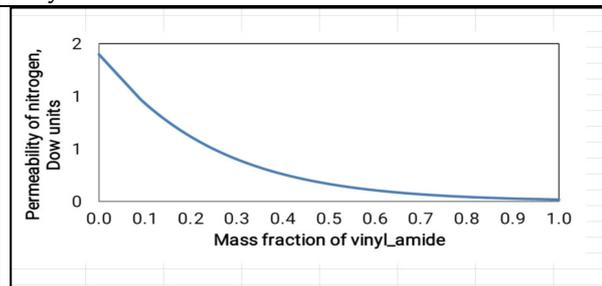
Figure 16. Change in the permeability of nitrogen with a mass fraction of vinyl amide.
