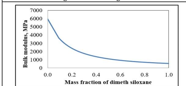
**Figure 5. Change in bulk modulus with mass fraction of dimethyl siloxane**
