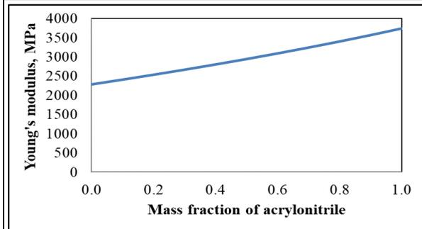
Figure 7. Change in Young's modulus with a mass fraction of acrylonitrile
