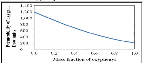
Figure 15. Change in permeability of oxygen with mass fraction of oxyphenyl
