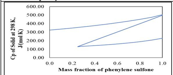
Figure 10. Change in heat capacity with mass fraction of phenylene sulfone.
