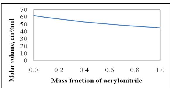
Figure 13. Change in molar volume with mass fraction of acrylonitrile.
