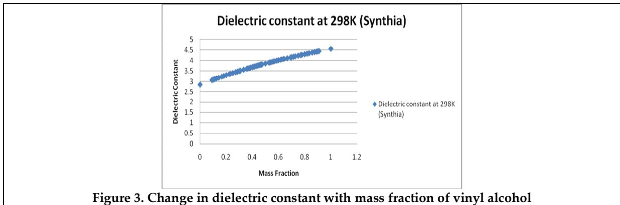
**Figure 3. Change in dielectric constant with mass fraction of vinyl alcohol**
