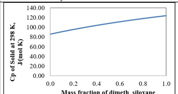
Figure 10. Change in heat capacity with mass fraction of dimethyl siloxane
