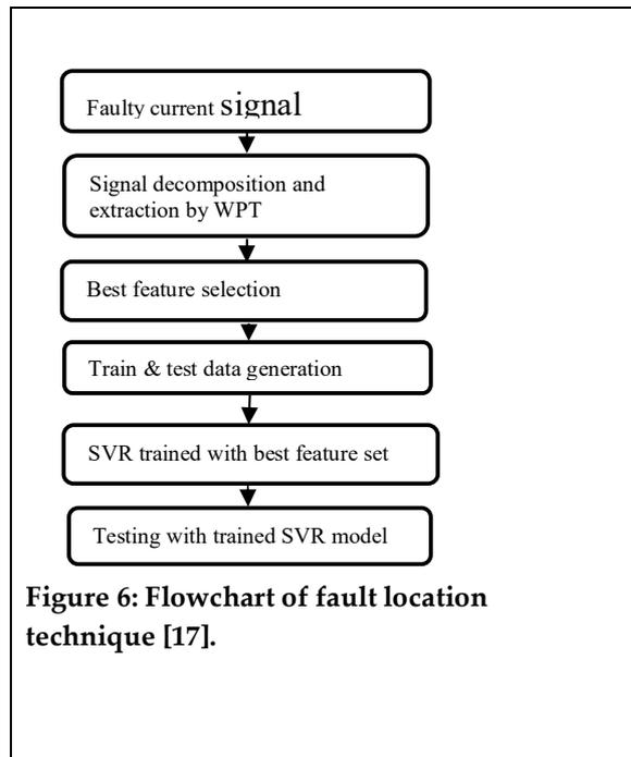
Figure 6: Flowchart of fault location technique [17].
