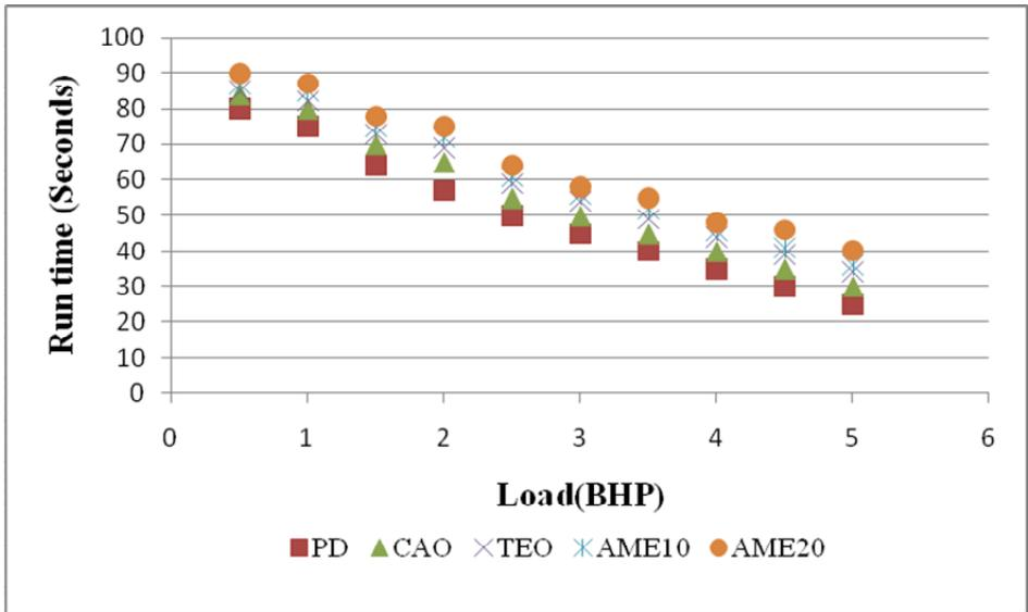
Fig. 2(a). Engine run-times for 20 ml oil at different load factor
