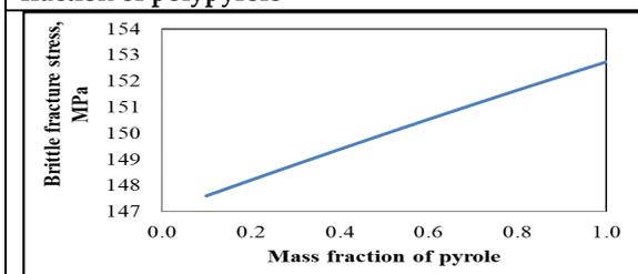
Figure 9. Change in brittle fracture stress with mass fraction of polypyrole
