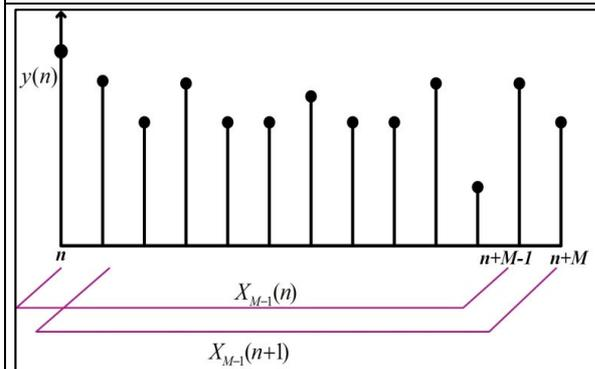
Fig. 3: Time-staggered, overlapping windows used by the LS/TLS ESPRIT algorithm
