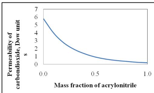
Figure 17. Change in the permeability of carbon dioxide with a mass fraction of acrylonitrile.
