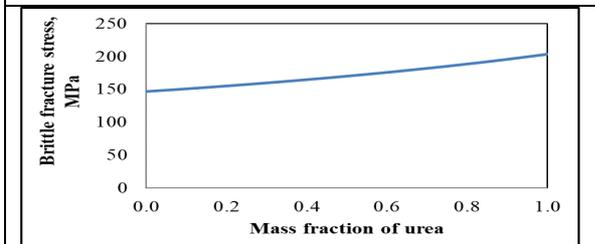
**Figure 9. Change in brittle fracture stress with mass fraction of Urea**
