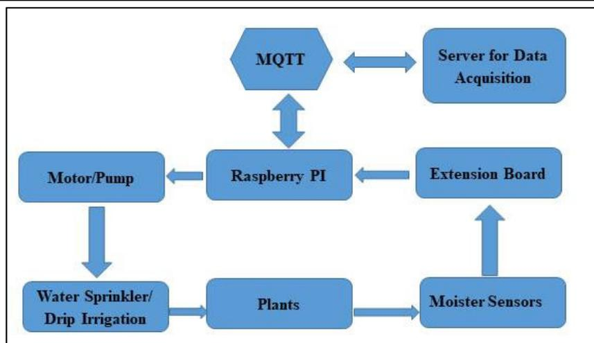
Figure 3: Raspberry Pi based smart irrigation system
