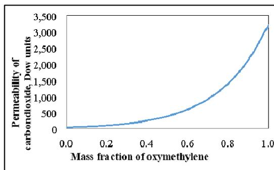
Figure 17. Change in permeability of carbon dioxide with mass fraction of polyoxymethylene
