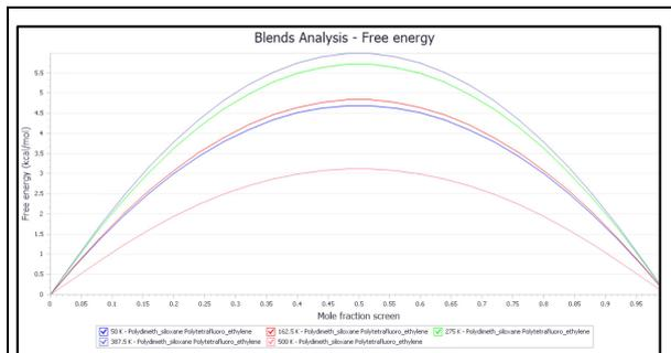
**Figure 1. Free energy change with mole fraction of polytetrafluoroethylene at different temperatures**
