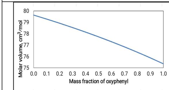
Figure 13. Change in molar volume with mass fraction of oxyphenyl
