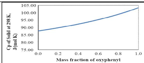
Figure 10. Change in heat capacity with mass fraction of oxyphenyl
