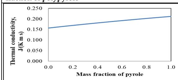
Figure 11. Change in thermal conductivity with mass fraction of polypyrole
