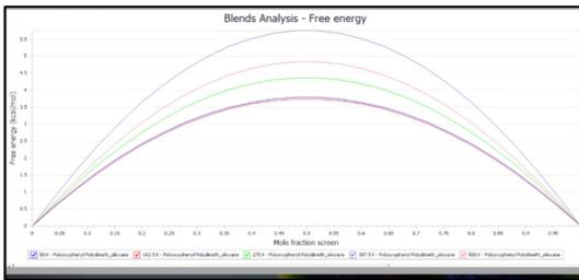
Figure 1. Free energy change with mole fraction of polydimeth\_siloxane at different temperatures
