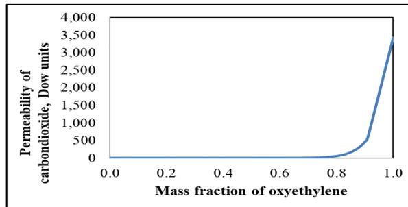
Figure 17. Change in permeability of carbon dioxide with mass fraction of oxyethylene
