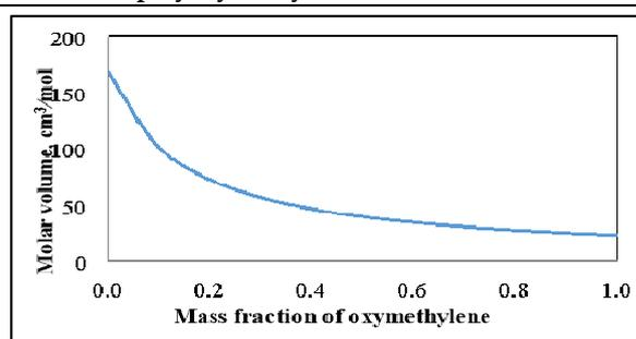
Figure 13. Change in molar volume with mass fraction of polyoxymethylene
