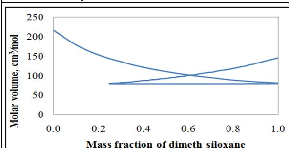
Figure 13. Change in molar volume with mass fraction of dimethylsiloxane
