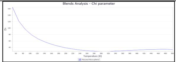
**Figure 2. Change in  $\chi$  (chi) value with temperature**
