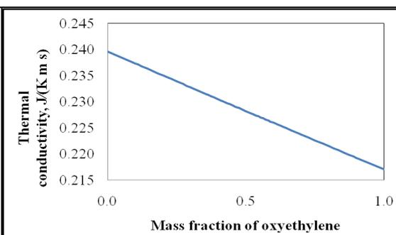
**Fig. 2. Change in thermal conductivity with mass fraction of oxyethylene**
