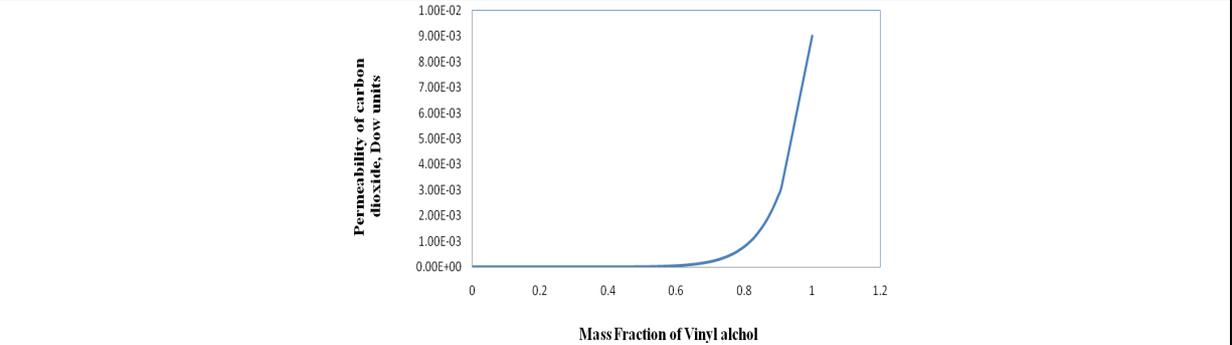
(Figure 5. Change in permeability of carbon dioxide with mass fraction of Vinyl Alcohol)
