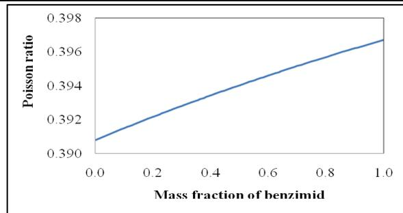
Fig.4. Change in Poisson modulus with mass fraction of Benzimid
