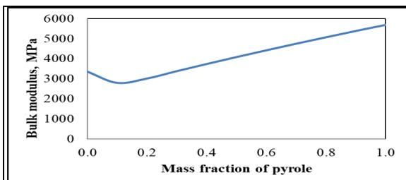
Figure 5. Change in bulk modulus with mass fraction of polypyrole
