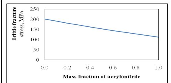
Figure 9. Change in brittle fracture stress with mass fraction of acrylonitrile.
