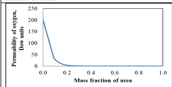
Figure 11. Change in permeability of oxygen with mass fraction of Urea
