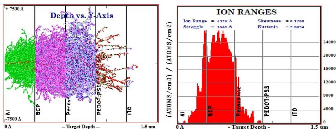
Fig.1.(Left) The passage of ion inside the perovskite based solar cell. Different colors indicate the passage of radiation at different layers. One can see that the ion will completely stop in the cell. (Right) the 1D histogram of the range of the ion which is nearly a gaussian distribution and the spread will tell the stragglings.
