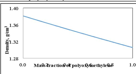
Figure 14. Change in density with mass fraction of polyoxymethylene
