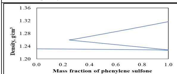
Figure 14. Change in density with mass fraction of phenylene sulfone.
