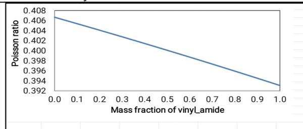
Figure 8. Change in Poisson modulus with a mass fraction of vinyl amide
