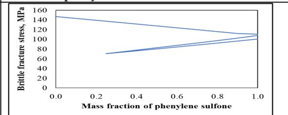
Figure 9. Change in brittle fracture stress with mass fraction of phenylene sulfone
