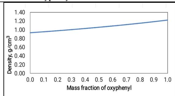
Figure 14. Change in density with mass fraction of oxyphenyl
