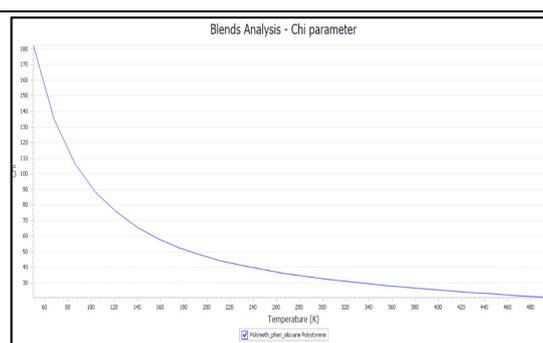
Figure 2. Change in  $\chi$  (chi) value with temperature
