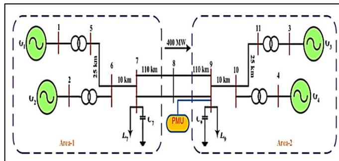
Fig 9.Single line schematic of two-area kundur's power system
