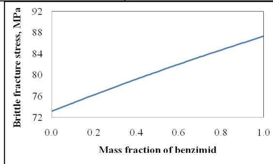
Fig. 5. Change in brittle fracture stress with mass fraction of Benzimid
