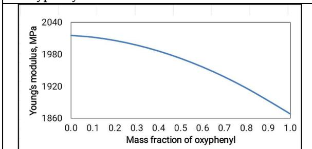
Figure 7. Change in Young's modulus with mass fraction of oxyphenyl
