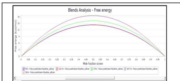
**Figure 1. Free energy change with mole fraction of polyether sulfone at different temperatures**
