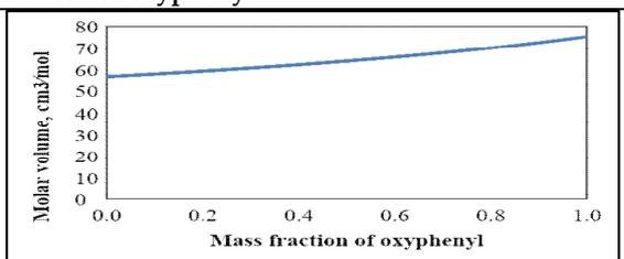
Figure 13. Change in molar volume with mass fraction of oxyphenyl
