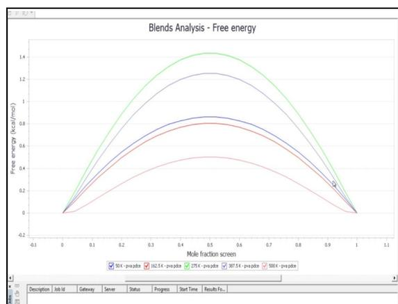
**Figure 1. Free energy change with mole fraction of Dichloroethylene at different temperatures**
