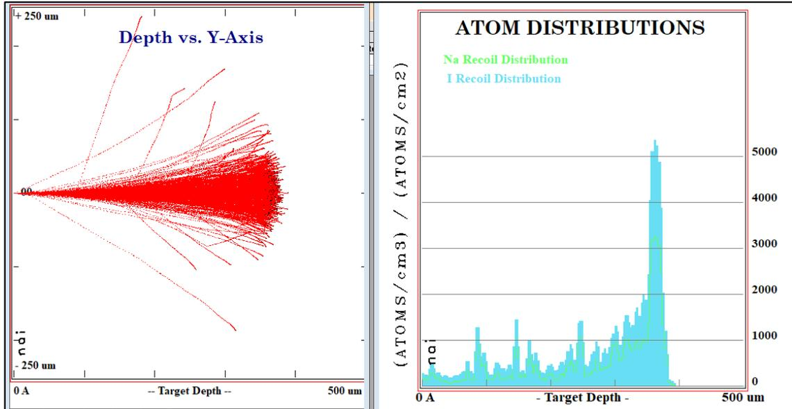
Fig.1. (Left) The range and the tracks of the Proton ion having 6 MeV incident energy inside NaI detector. (Right) same incident ion but the recoil distribution.
