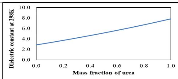
Figure 13. Change in dielectric constant with mass fraction of Urea
