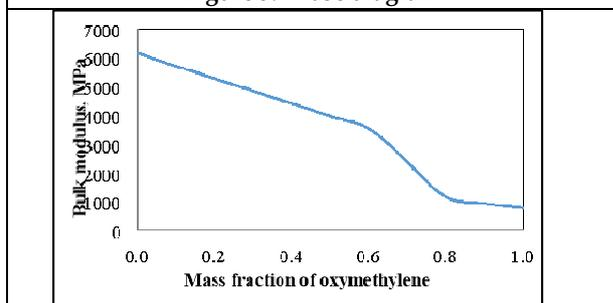
**Figure 5. Change in bulk modulus with mass fraction of polyoxymethylene**
