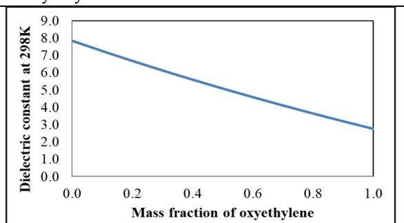
Figure 12. Change in dielectric constant with mass fraction of oxyethylene
