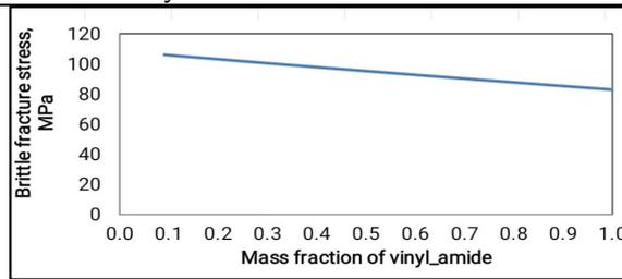
Figure 9. Change in brittle fracture stress with a mass fraction of vinyl amide
