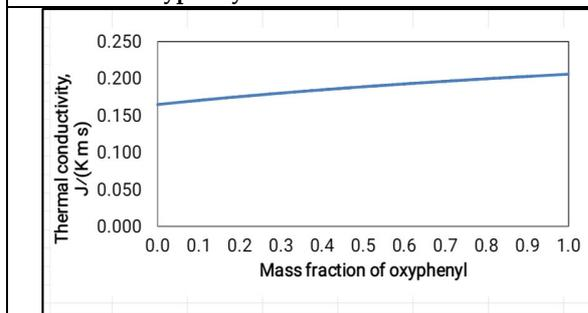
Figure 11. Change in thermal conductivity with mass fraction of oxyphenyl
