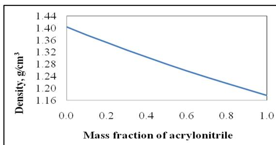
Figure 14. Change in density with a mass fraction of acrylonitrile.
