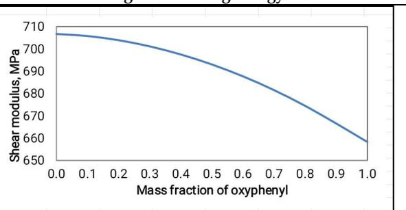
Figure 6. Change in shear modulus with mass fraction of oxyphenyl
