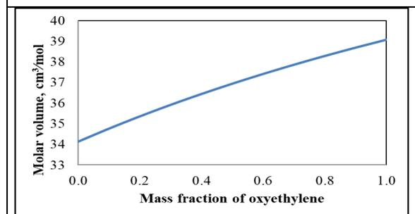
Figure 13. Change in molar volume with mass fraction of oxyethylene
