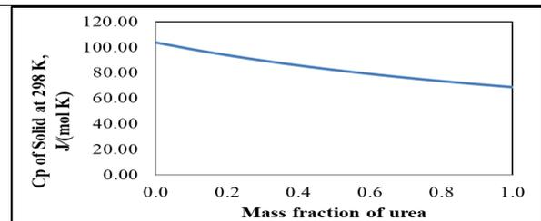
**Figure 10. Change in heat capacity with mass fraction of Urea**
