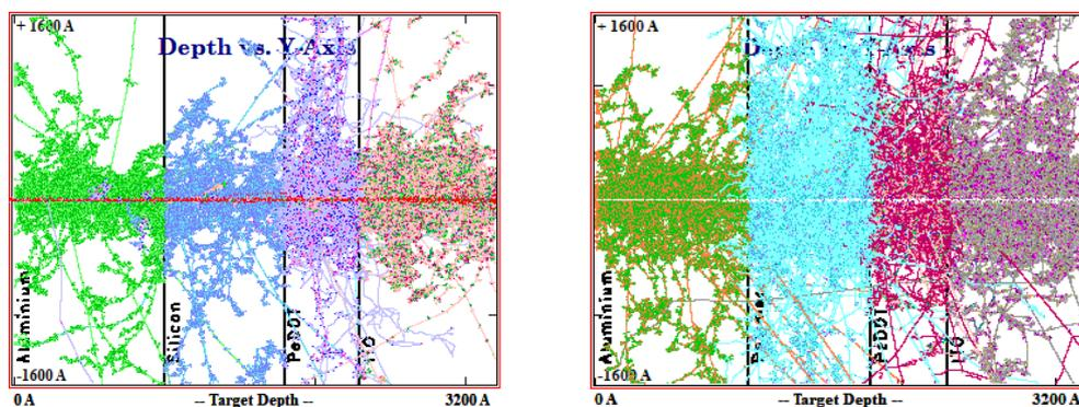
Fig. 2. The TRIM calculation for standard Silicon detector which shows the distribution of the energy loss spread (Left). The same energy loss spread for proposed ITO based semiconductor. One can see that the track is narrow in conventional Silicon whereas wide spread in the proposed ITO (Right).
