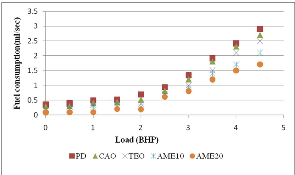
Fig. 2(b). Fuel consumption per second at different load factor
