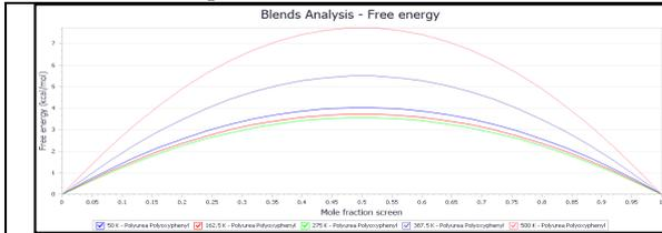
**Figure 1. Free energy change with mole fraction of Urea at different temperatures**
