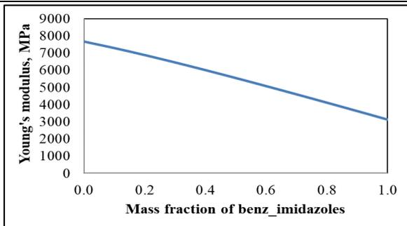
Figure 7. Change in Young's modulus Vs mass fraction of Benzimidazole.
