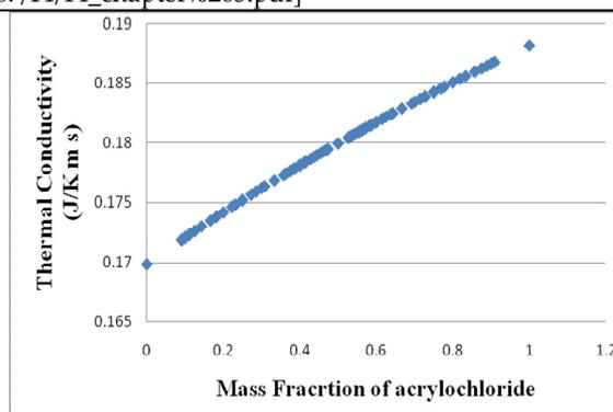
Figure 2. Variation in thermal conductivity with mass fraction of acrylochloride
