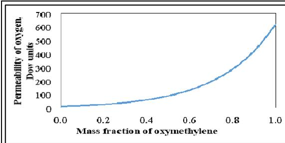
Figure 15. Change in permeability of oxygen with mass fraction of polyoxymethylene
