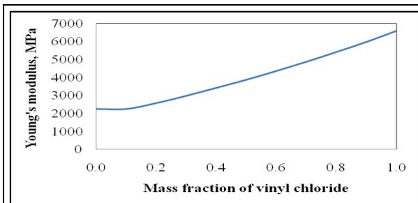
Figure 7. Change in Young's modulus with mass fraction of vinyl chloride.
