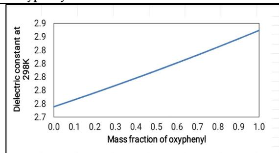
Figure 12. Change in dielectric constant with mass fraction of oxyphenyl
