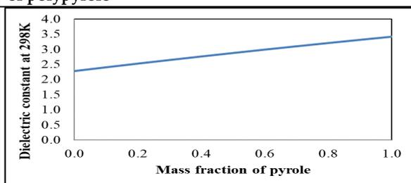
Figure 12. Change in dielectric constant with mass fraction of polypyrole
