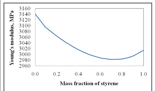
**Figure 7: Change in Young's modulus with mass fraction of styrene**
