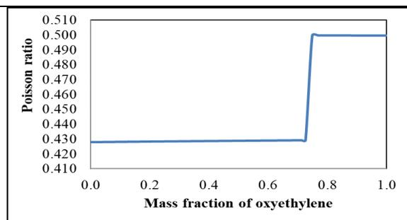
Figure 8. Change in Poisson modulus with mass fraction of oxyethylene
