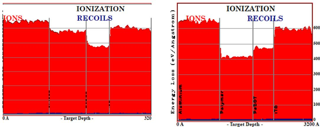
Fig.1. The same TRIM calculation for newly proposed semiconductor. The generation of the electron and hole are nearly same in both. A small increase can be seen in Si based detector which is expected (Left). The proposed ITO based semiconductor. One can see the ionization recoil spectra are almost same for the both the types of detector which indicates the applicability of the ITO based detector (Right).
