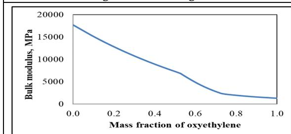
**Figure 5. Change in bulk modulus with mass fraction of oxyethylene**
