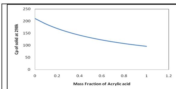
Figure 1. Change in heat capacity with mass fraction of Acrylic acid
