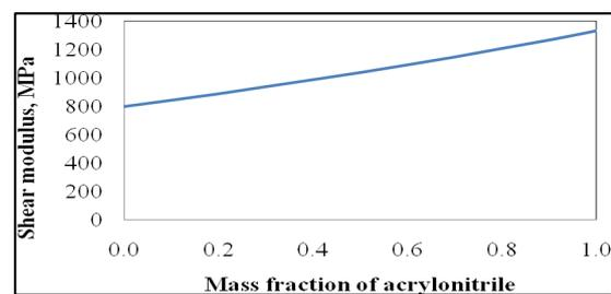
Figure 6. Change in shear modulus with mass fraction of acrylonitrile
