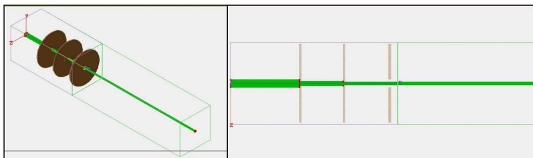
Fig.2.The 3D view of the metallic disc used for the simulation (left). The cross sectional view of the same (Right)
