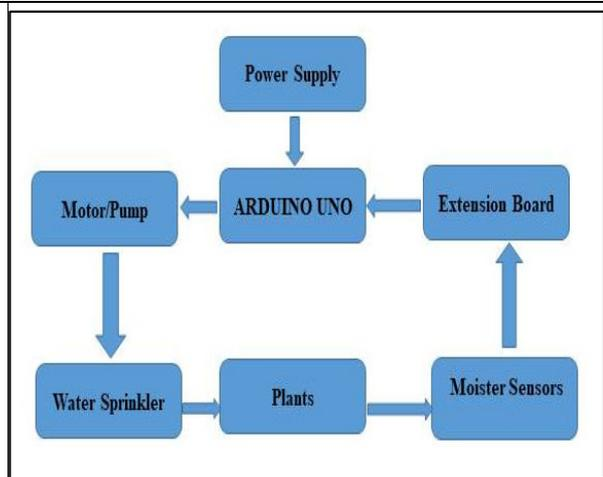
Figure 2. Arduino based smart irrigation system
