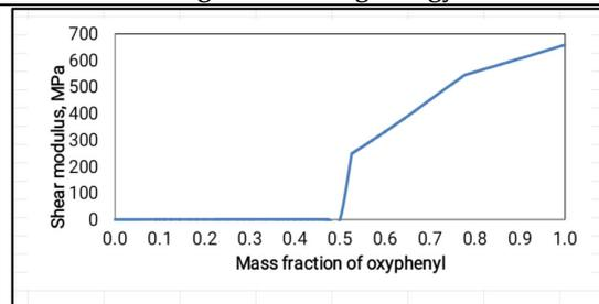
Figure 6. Change in shear modulus with mass fraction of oxyphenyl
