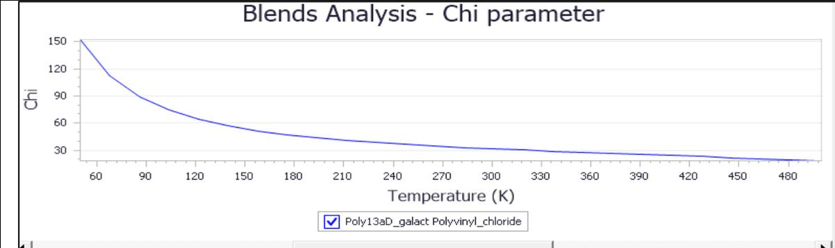
**Figure 2. Change in  $\chi$  (chi) value with temperature**
