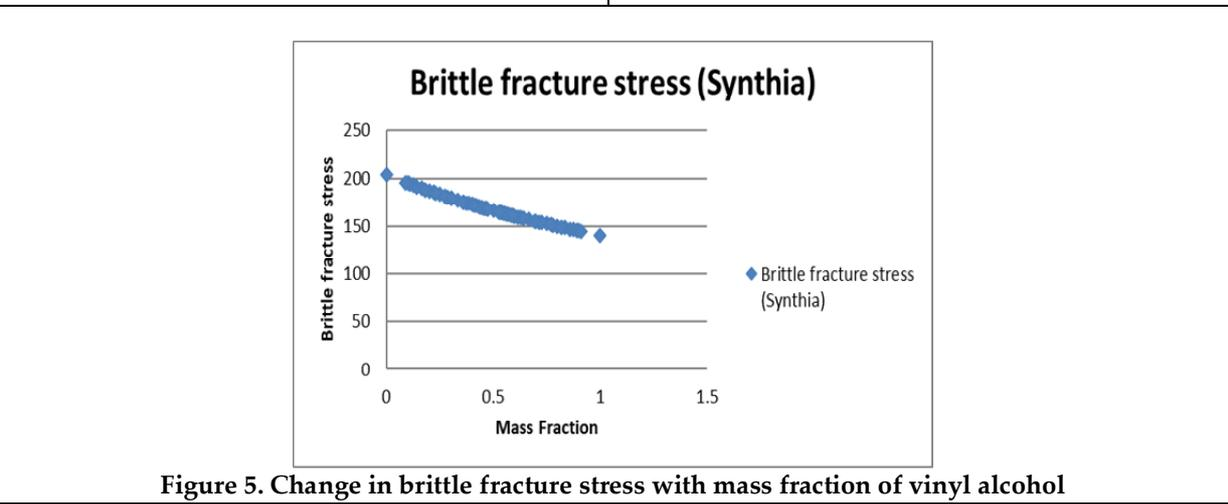
Figure 5. Change in brittle fracture stress with mass fraction of vinyl alcohol
