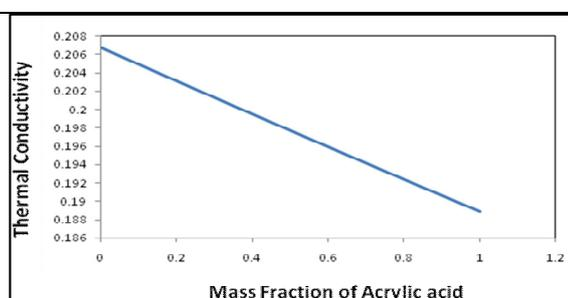
Figure 2. Change in thermal conductivity with mass fraction of Acrylic acid
