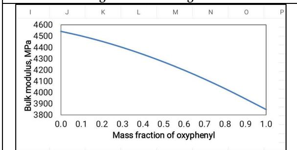
Figure 5. Change in bulk modulus with mass fraction of oxyphenyl
