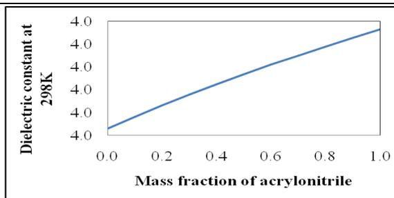
Figure 12. Change in dielectric constant with a mass fraction of acrylonitrile.
