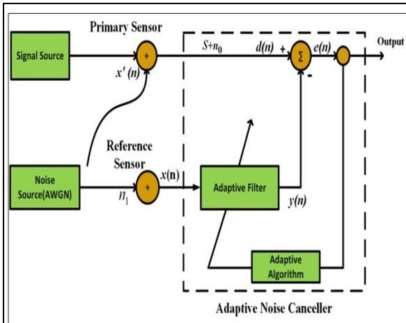
Fig. 1: Adaptive LMSSS filter for noise cancellation
