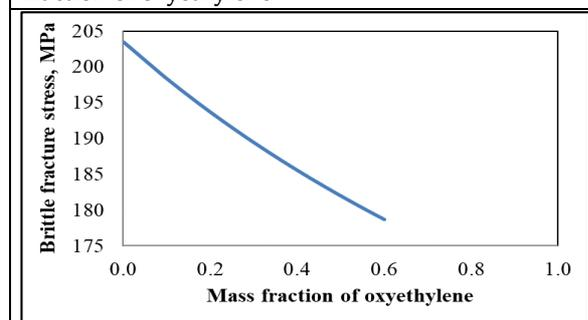
Figure 9. Change in brittle fracture stress with mass fraction of oxyethylene
