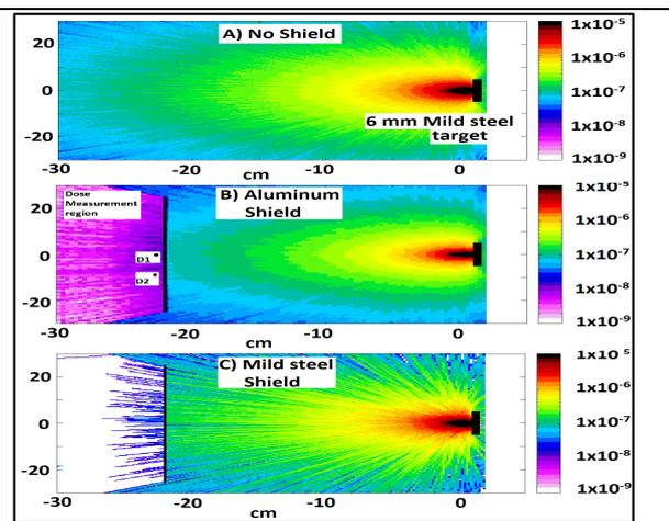
Fig 2. Photon distribution produced due to 50 keV electrons impinging on Mild steel target
