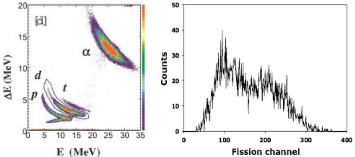
Fig.1. (Left) The identification of the charge radiation using the silicon detector. Each light particle is very clearly seperable. Here the detector looks like in the telescope arrangement (see text for details). (Right) Same detector used for fission, no such particle identification for fission and also the plasma effect makes the detector bad [3,4].
