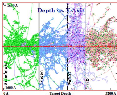
**Fig.2.The TRIM calculation for standard Silicon detector which shows the distribution of the energy loss spread. When a charge particle move inside the SSBsemiconductor detector. One can see that the tracks are spread over the full range which is not the case for gas detector.**
