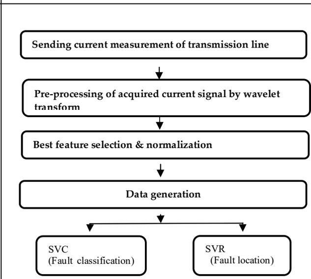
**Figure 5. Block diagram of SVM based fault classification and location in a transmission line. [19].**
