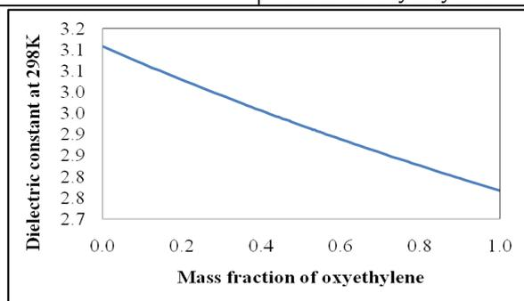
**Fig. 3. Change in dielectric constant with mass fraction of oxyethylene**
