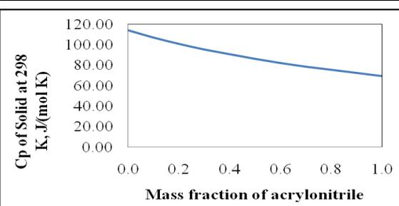
Figure 10. Change in heat capacity with a mass fraction of acrylonitrile.
