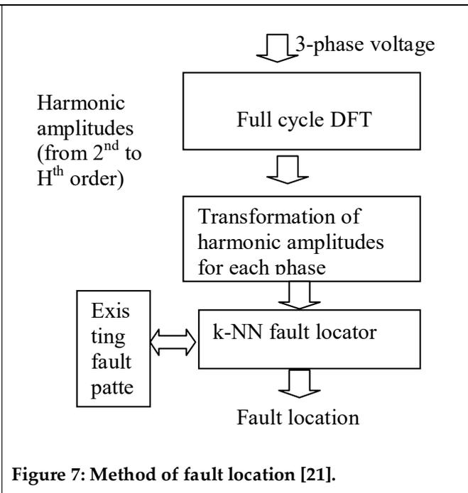
Figure 7: Method of fault location [21].
