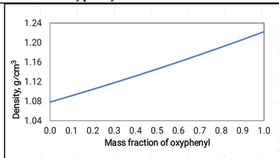
Figure 14. Change in density with mass fraction of oxyphenyl
