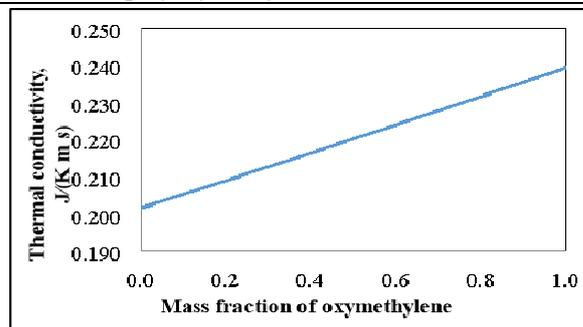
Figure 11. Change in thermal conductivity with mass fraction of polyoxymethylene
