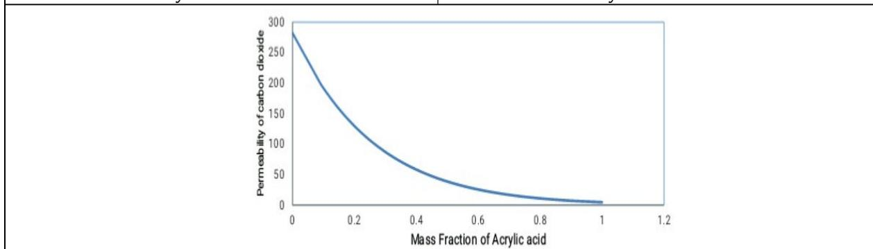
Figure 5. Change in permeability of carbon dioxide with mass fraction of acrylic acid
