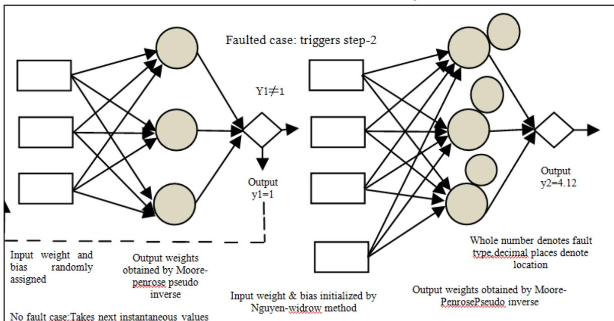
**Figure 1. Schematic representation of the proposed fault diagnosis method [13].**
