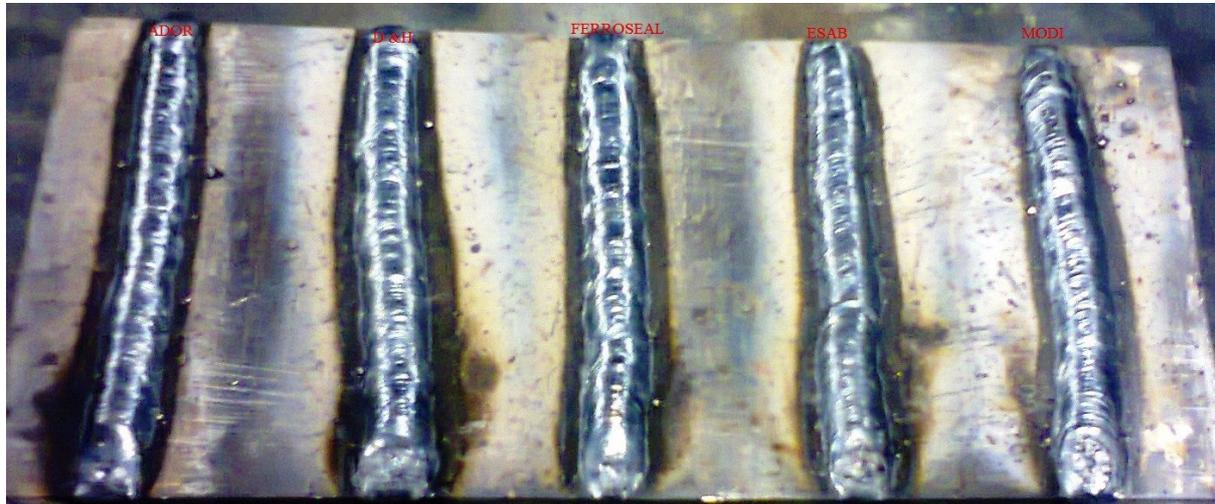
Fig. 8 Welded beads by five types of electrodes
