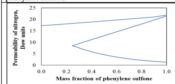
Figure 16. Change in permeability of nitrogen with mass fraction of phenylene sulfone.
