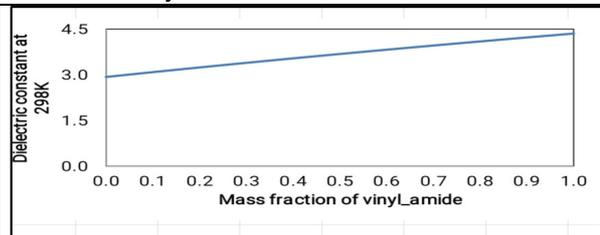
Figure 12. Change in dielectric constant with the mass fraction of vinyl amide
