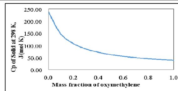
Figure 10. Change in heat capacity with mass fraction of polyoxymethylene
