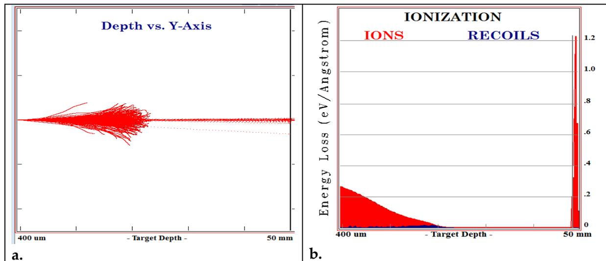
**Fig.1. (a) the TRIM calculation for standard P-10 gas using the proton of energy 50 MeV (the straight thin line) and the thick broadening is for 50 MeV <sup>120</sup>Sn heavy ion. (b) The ions and recoils distribution within the gas volume for both ions.**
