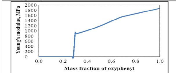
**Figure 7. Change in Young's modulus with mass fraction of oxyphenyl**
