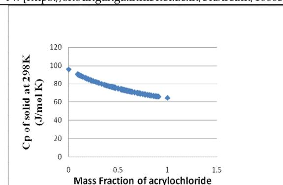
Figure 1. Variation in heat capacity with mass fraction of acrylochloride
