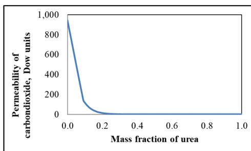
Figure 16. Change in permeability of carbon dioxide with mass fraction of Urea
