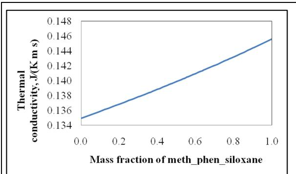
Figure 11. Change in thermal conductivity with mass fraction of polymethyl phenyl siloxane
