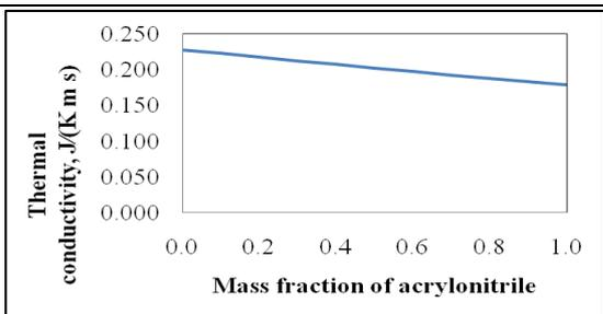
Figure 11. Change in thermal conductivity with mass fraction of acrylonitrile.
