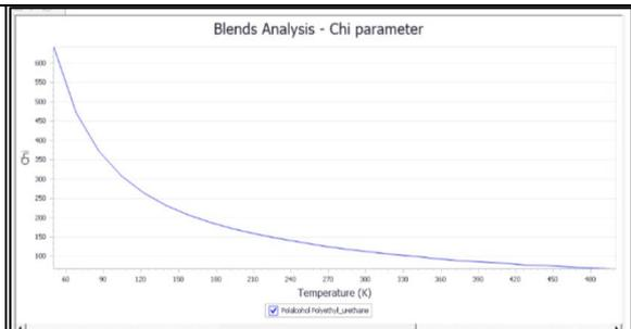
Figure 2. Change in  $\chi$  (chi) value with temperature
