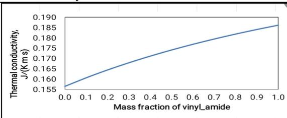
Figure 11. Change in thermal conductivity with the mass fraction of vinyl amide
