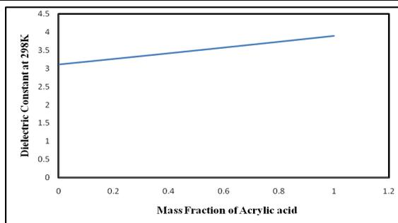
Figure 3. Change in dielectric constant with mass fraction of acrylic acid
