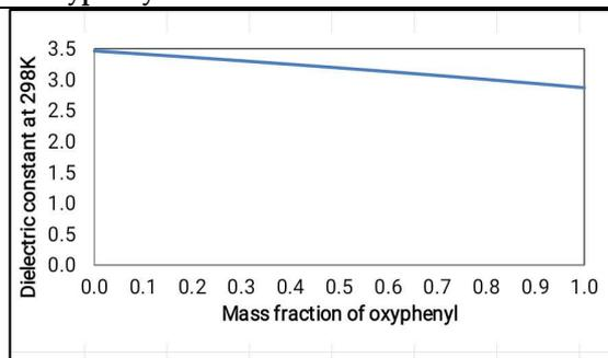
Figure 12. Change in dielectric constant with mass fraction of oxyphenyl
