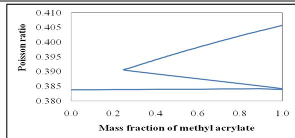
Figure 8. Change in Poisson modulus with mass fraction of acrylic acid
