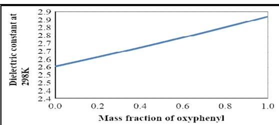
Figure 12. Change in dielectric constant with mass fraction of oxyphenyl
