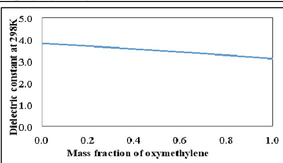
Figure 12. Change in dielectric constant with mass fraction of polyoxymethylene
