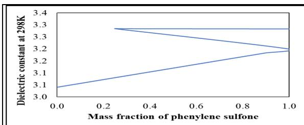
Figure 12. Change in dielectric constant with mass fraction of phenylene sulfone.
