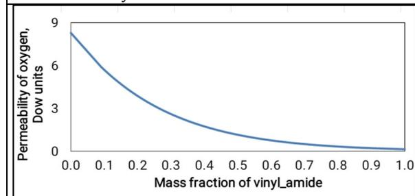
Figure 15. Change in the permeability of oxygen with a mass fraction of vinyl amide
