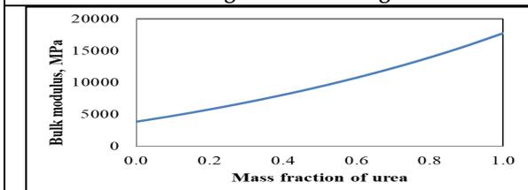
**Figure 5. Change in bulk modulus with mass fraction of Urea**
