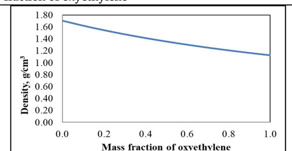
Figure 14. Change in density with mass fraction of oxyethylene
