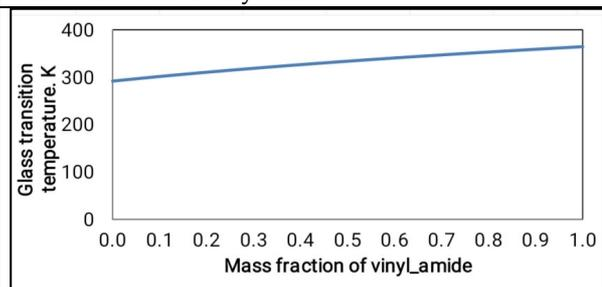
Figure 18. Change in the glass transition temperature with the mass fraction of vinyl amide
