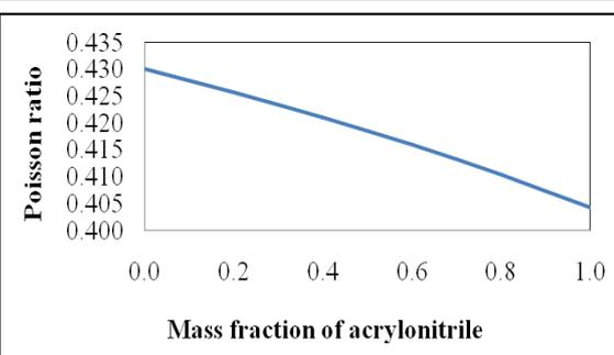
Figure 8. Change in Poisson modulus with mass fraction of acrylonitrile
