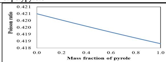
Figure 8. Change in Poisson modulus with mass fraction of polypyrole
