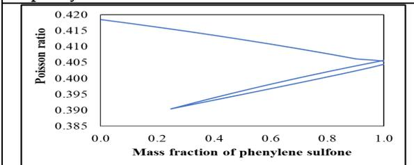
Figure 8. Change in Poisson modulus with mass fraction of phenylene sulfone.
