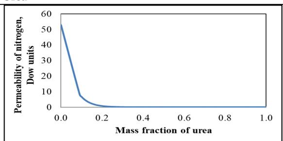
Figure 12. Change in permeability of nitrogen with mass fraction of Urea
