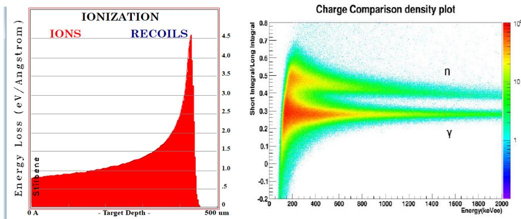
Figure 3. (left) Bragg's curve and the full energy loss (right) the pulse shape analysis and the identification of the gamma and neutron.
