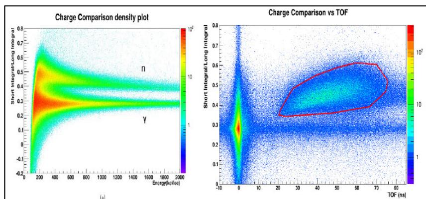
Fig 1. (Left) The Pulse shape discrimination method and (Right) TOF analysis of the previous data using the newly developed algorithm. Neutron and the gamma are very well separated from both the figure.
