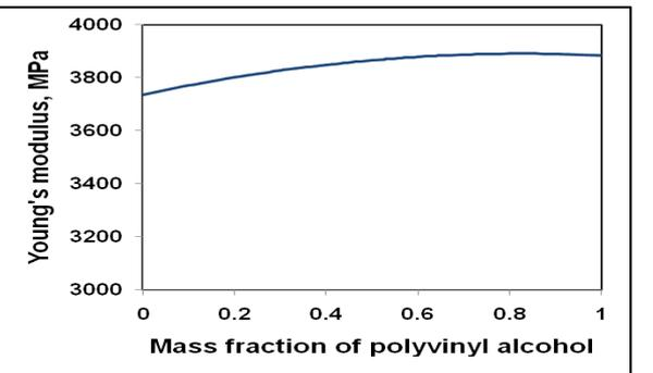
Figure3. Change in Young's modulus with the mass fraction of vinyl alcohol
