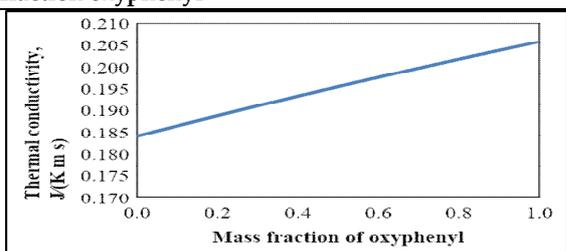
Figure 11. Change in thermal conductivity with mass fraction of oxyphenyl
