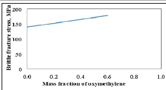
Figure 9. Change in brittle fracture stress with mass fraction of polyoxymethylene
