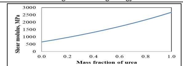
**Figure 6. Change in shear modulus with mass fraction of Urea**
