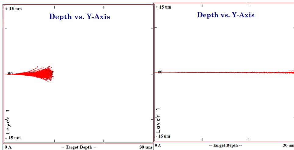
Fig.2. (left) The heavy ion (fission fragement) from the reaction  ${}^6\text{Li}+{}^{209}\text{Bi}$  at 40 MeV is passing through the SSB(silicon surface barrier ) detector and the range is very less i.e. all the ions will stop there and creat a pulse height defect. (Right) The same expriment but the emitted particle (alpha) is passing through the detctor. In both of the cases the enegy of the particle is same.
