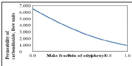
Figure 17. Change in permeability of carbon dioxide with mass fraction of oxyphenyl
