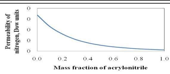
Figure 16. Change in the permeability of nitrogen with a mass fraction of acrylonitrile.
