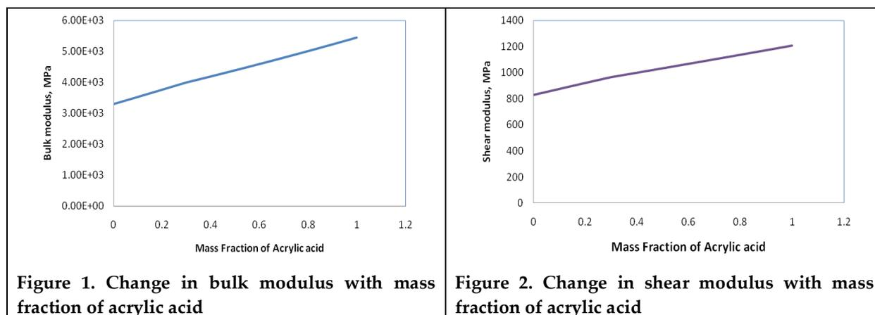
**Figure 1. Change in bulk modulus with mass fraction of acrylic acid**
