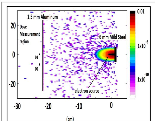
Fig.1. Secondary electron distribution due to mono energetic 50 keV p beam.
