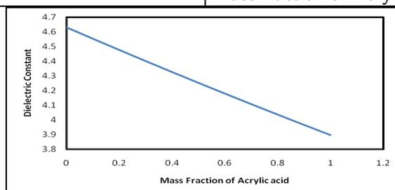
Figure 3. Change in dielectric constant with mass fraction of Acrylic acid
