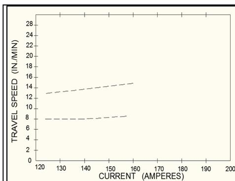
Fig. 6. Travel speed Vs Current (E6013 SMAW electrode)
