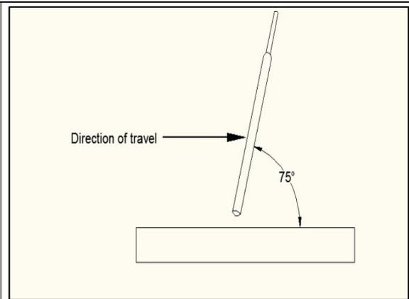
Fig. 4. Suitable angle for flat welding for SMAW
