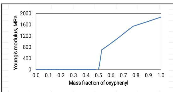
Figure 7. Change in Young's modulus with mass fraction of oxyphenyl
