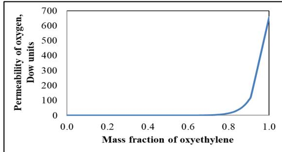
Figure 15. Change in permeability of oxygen with mass fraction of oxyethylene
