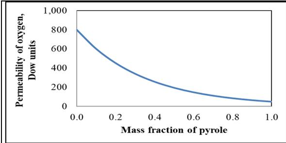
Figure 15. Change in permeability of oxygen with mass fraction of polypyrole
