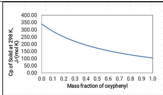
Figure 10. Change in heat capacity with mass fraction of oxyphenyl
