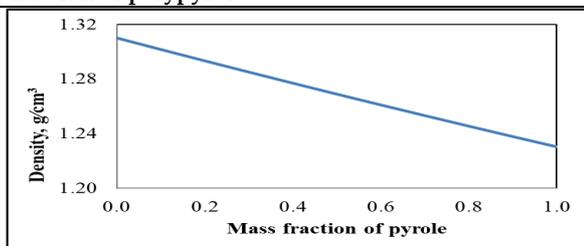
Figure 14. Change in density with mass fraction of polypyrole
