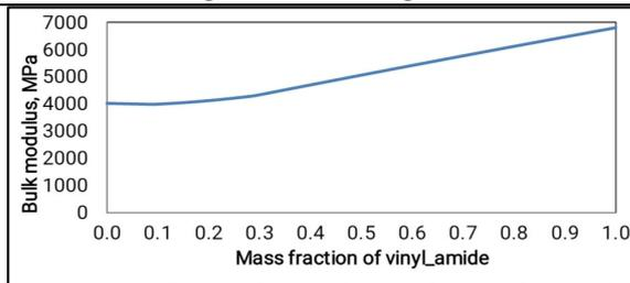
Figure 5. Change in bulk modulus with the mass fraction of Vinyl amide
