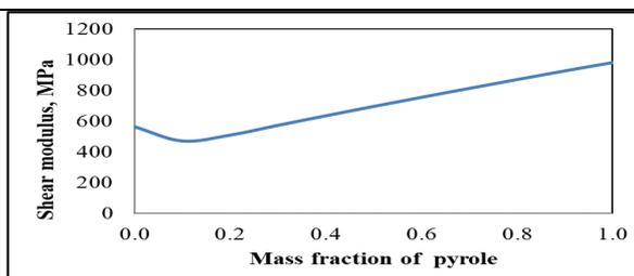
Figure 6. Change in shear modulus with mass fraction of polypyrole
