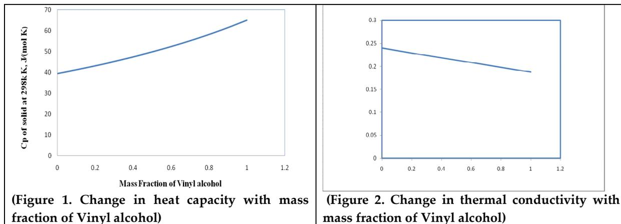
(Figure 1. Change in heat capacity with mass fraction of Vinyl alcohol)
