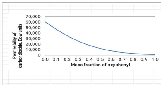
Figure 17. Change in permeability of carbon dioxide with mass fraction of oxyphenyl
