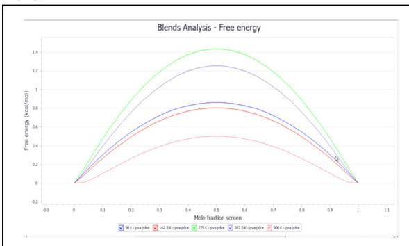
**Figure 1. Free energy change with mole fraction of Polydichloroethylene incorporated at different temperature**
