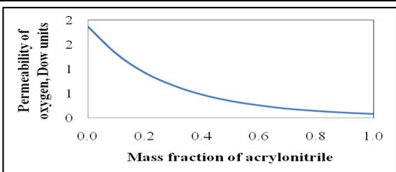
Figure 15. Change in the permeability of oxygen with a mass fraction of acrylonitrile.
