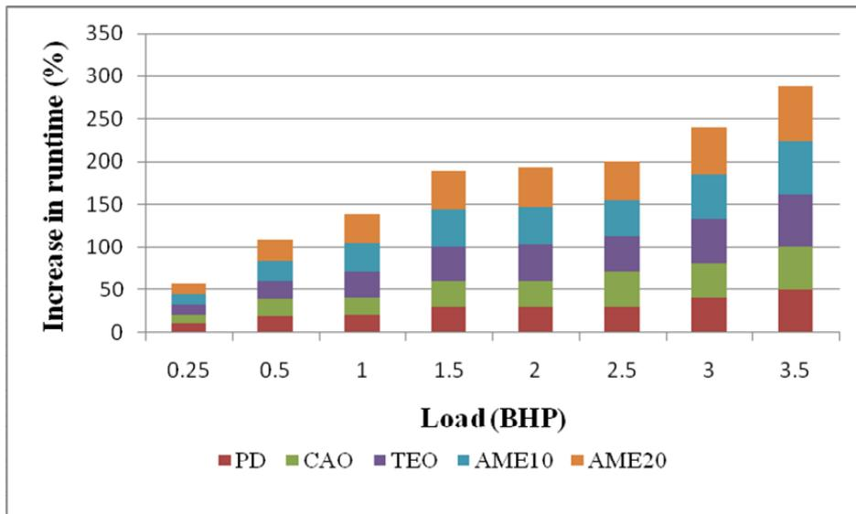
Fig. 3. Percent increase in run-time for different oils at variable load.
