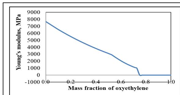
Figure 7. Change in Young's modulus with mass fraction of oxyethylene
