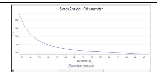
**Figure 2 Change in  $\chi$  (chi) value with temperature**
