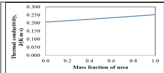
Figure 11. Change in thermal conductivity with mass fraction of Urea
