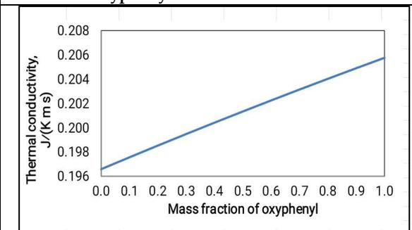
Figure 11. Change in thermal conductivity with mass fraction of oxyphenyl
