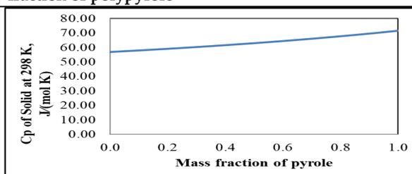
Figure 10. Change in heat capacity with mass fraction of polypyrole
