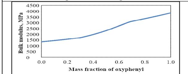
**Figure 5. Change in bulk modulus with mass fraction of oxyphenyl**
