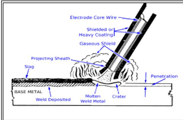
Fig. 3. Welding Operation
