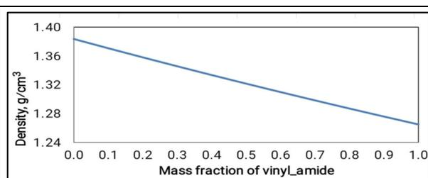
Figure 14. Change in density with the mass fraction of vinyl amide
