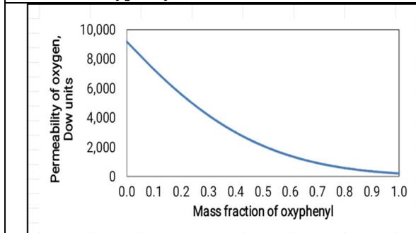
Figure 15. Change in permeability of oxygen with mass fraction of oxyphenyl
