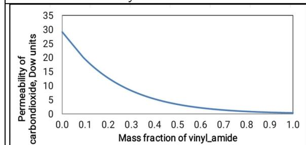
Figure 17. Change in the permeability of carbon dioxide with a mass fraction of vinyl amide
