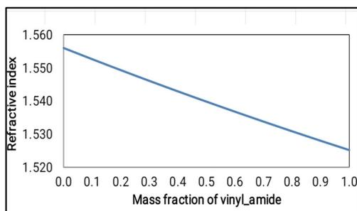
Figure 19. The graph between the refractive Index and the mass fraction of vinyl amide.
