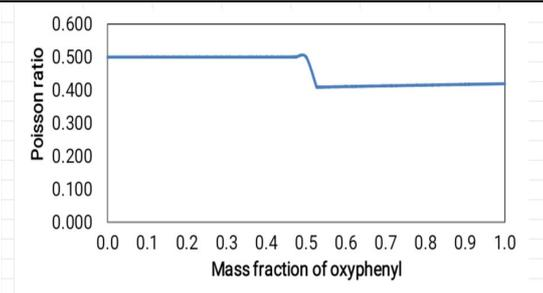
Figure 8. Change in Poisson modulus with mass fraction of oxyphenyl
