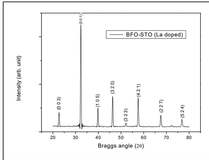
Figure 1. Indexed XRD pattern of La doped BFST
