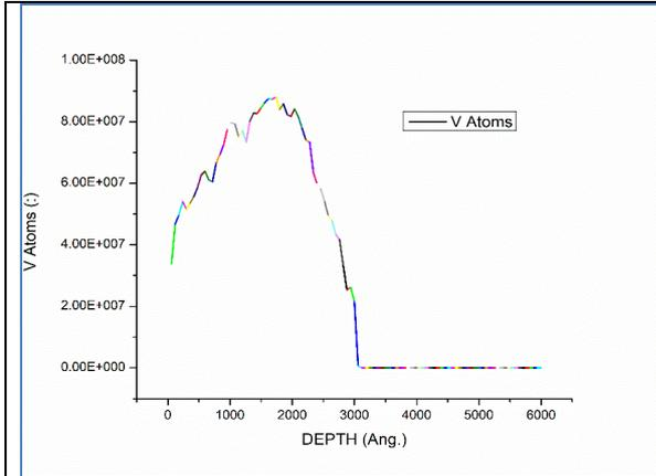
Fig.2.Variation of vanadium atoms with penetration depth
