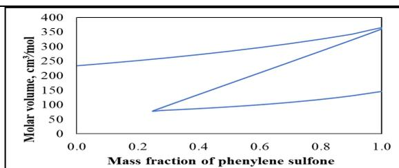
Figure 13. Change in molar volume with mass fraction of phenylene sulfone.
