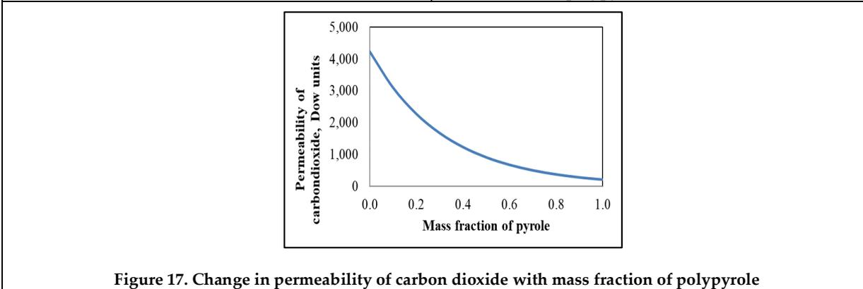
Figure 17. Change in permeability of carbon dioxide with mass fraction of polypyrole
