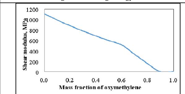
**Figure 6. Change in shear modulus with mass fraction of polyoxymethylene**
