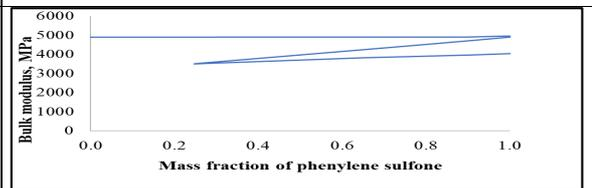
Figure 5. Change in bulk modulus with mass fraction of phenylene sulfone.
