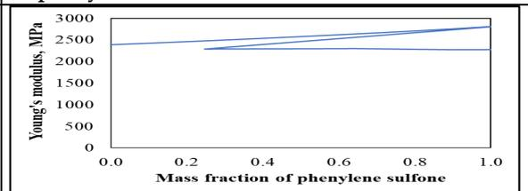
Figure 7. Change in Young's modulus with mass fraction of phenylene sulfone
