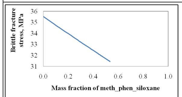
Figure 9. Change in brittle fracture stress with mass fraction of dimethyl siloxane
