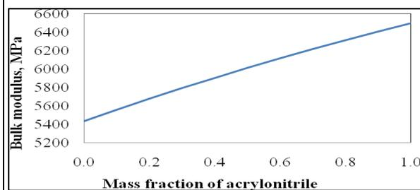
Figure 5. Change in bulk modulus with a mass fraction of acrylonitrile.
