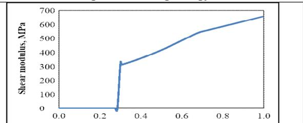
**Figure 6. Change in shear modulus with mass fraction of oxyphenyl**
