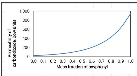
**Figure 17. Change in permeability of carbon dioxide with mass fraction of oxyphenyl**
