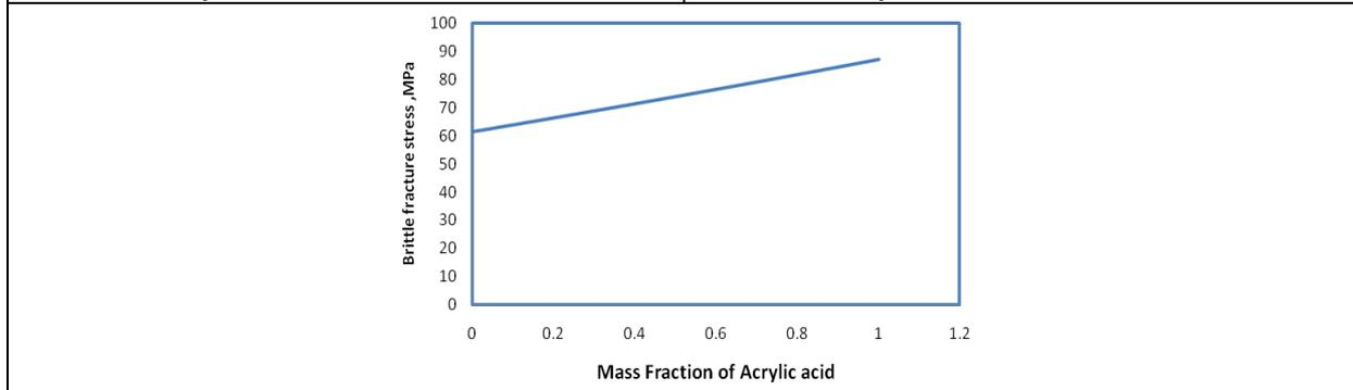
**Figure 5. Change in brittle fracture stress with mass fraction of acrylic acid**
