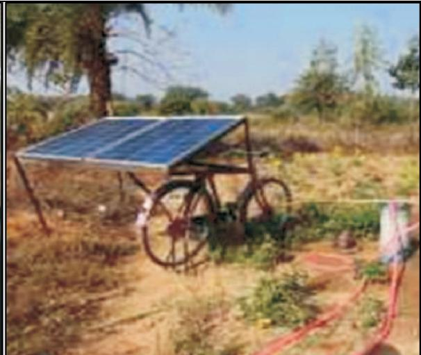
Figure 3. Cycle mounted solar powered irrigation system
