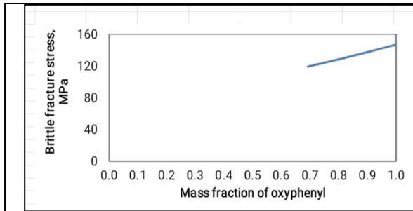
Figure 9. Change in brittle fracture stress with mass fraction of oxyphenyl
