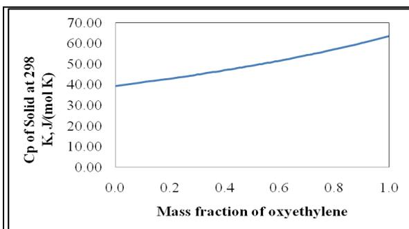
**Fig.1. Change in heat capacity with mass fraction of oxyethylene**
