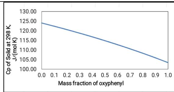
Figure 10. Change in heat capacity with mass fraction of oxyphenyl
