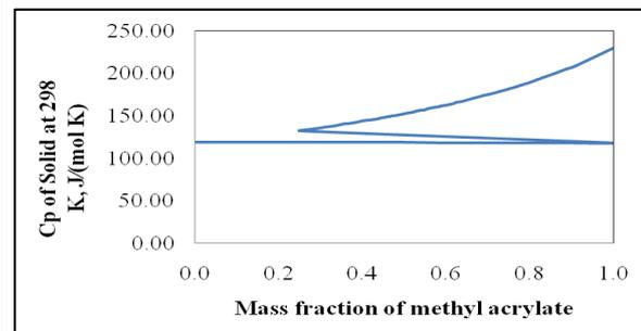
Figure 10. Change in heat capacity with mass fraction of acrylic acid
