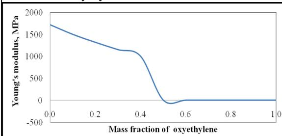
**Figure 7 Change in Young's modulus with mass fraction of oxyethylene**
