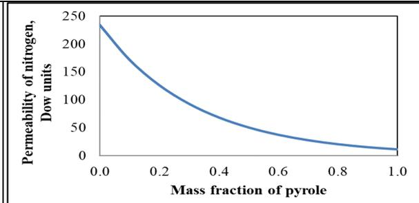
Figure 16. Change in permeability of nitrogen with mass fraction of polypyrole
