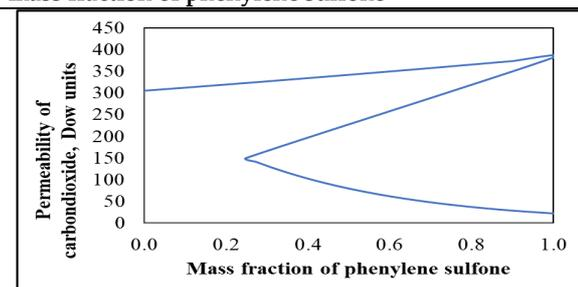
Figure 17. Change in permeability of carbon dioxide with mass fraction of phenylene sulfone.
