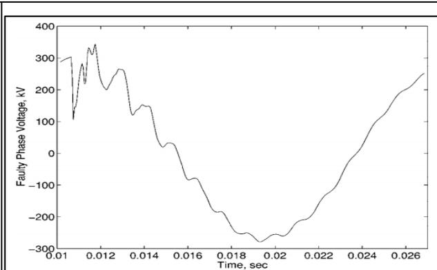
**Figure 3. Voltage Waveform of the faulty Phase [17]**
