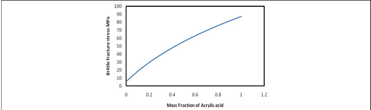
Figure 5. Change in brittle fracture stress with mass fraction of acrylic acid
