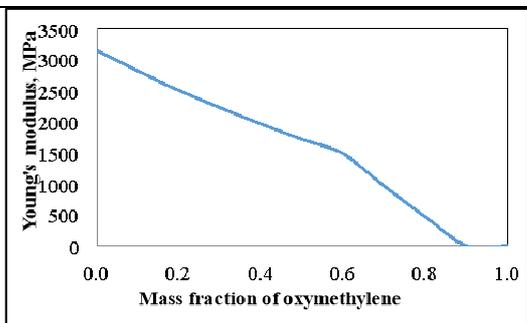
Figure 7. Change in Young's modulus with mass fraction of polyoxymethylene
