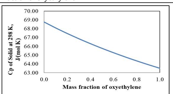
Figure 10. Change in heat capacity with mass fraction of oxyethylene
