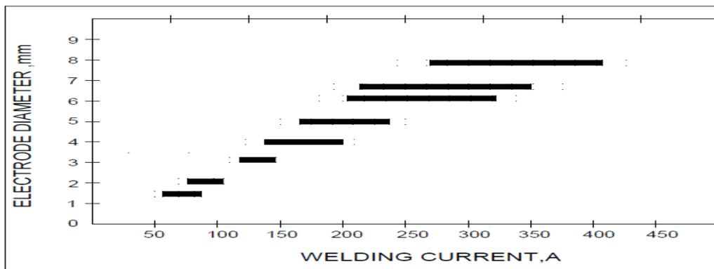
Fig. 5. Welding current for different diameter of electrode
