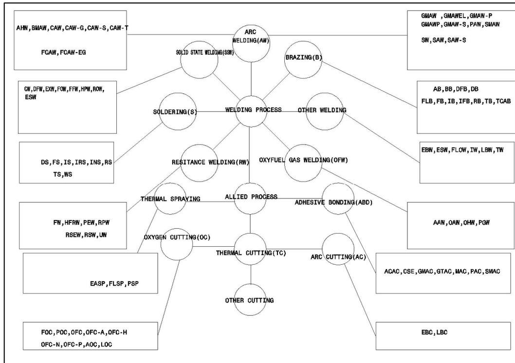
Fig. 1. Welding process classification
