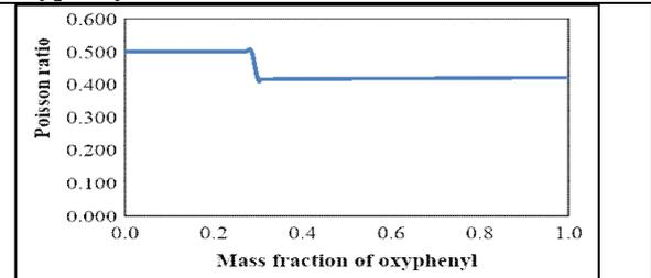
**Figure 8. Change in Poisson modulus with mass fraction of oxyphenyl**
