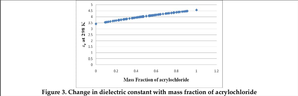
Figure 3. Change in dielectric constant with mass fraction of acrylochloride
