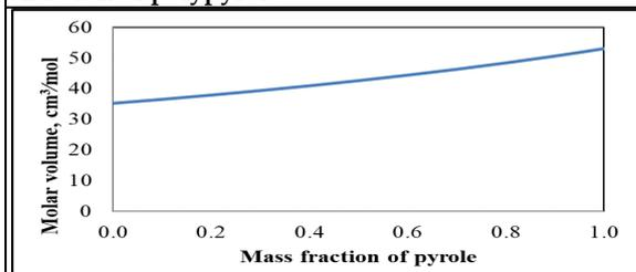
Figure 13. Change in molar volume with mass fraction of polypyrole
