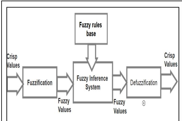
**Figure 2. Fuzzy Logic System Architecture.**
