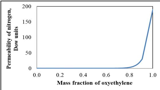
Figure 16. Change in permeability of nitrogen with mass fraction of oxyethylene
