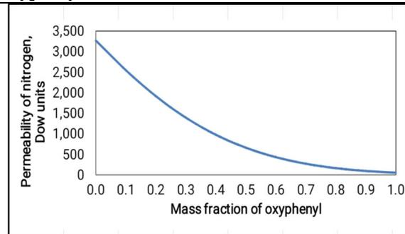
Figure 16. Change in permeability of nitrogen with mass fraction of oxyphenyl
