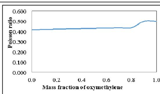
Figure 8. Change in Poisson modulus with mass fraction of polyoxymethylene
