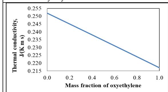
Figure 11. Change in thermal conductivity with mass fraction of oxyethylene
