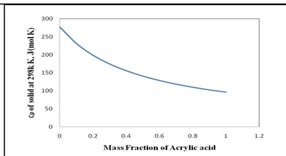
Figure 1. Change in heat capacity with mass fraction of acrylic acid
