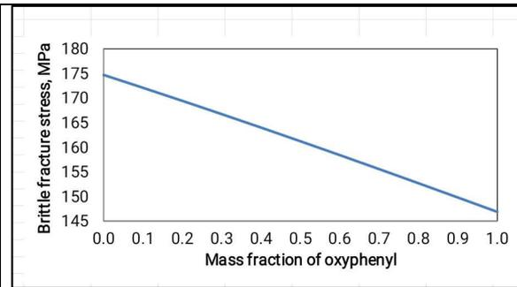
Figure 9. Change in brittle fracture stress with mass fraction of oxyphenyl
